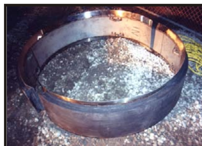
ABOVE: CUSTOM FABRICATED INTERNAL PIPE REPAIR BAND
