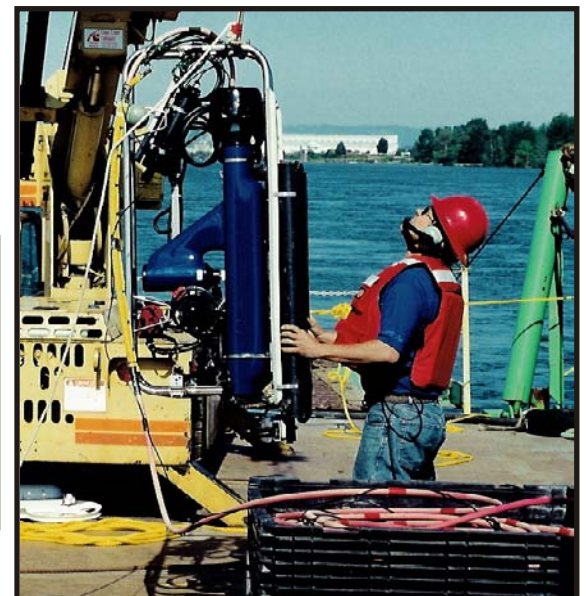
RIGHT: ROV RECOVERED AFTER DEPLOYMENT INTO THE OUTFALL SYSTEM (1750 ft. Penetration) TO PERFORM DIGITAL VIDEO AND DUAL IMAGING SONAR SURVEYS OF SEDIMENT PROFILE IN THE PIPE AND THE STRUCTURAL CONDITION OF EACH PIPE JOINT. (Accuracy +/- 1/8 inch)
